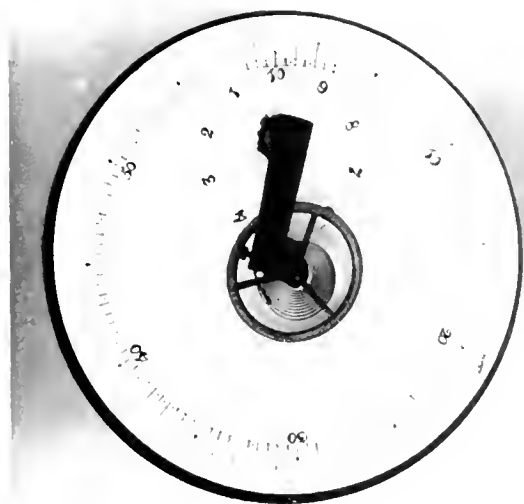
Figure 17. A TIMER DIAL that is probably either experimental or very early. Note that the fractions of a second (quarters) are shown on the outside dial instead of on a separate dial. This dial was converted at the factory for use as the base of a hairspring vibrating stand. A dial different from this but having the same arrangement of circles is known. (In author's collection.)
